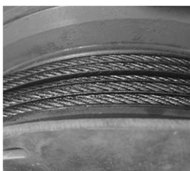
Figure 6. Wheel groove wear
