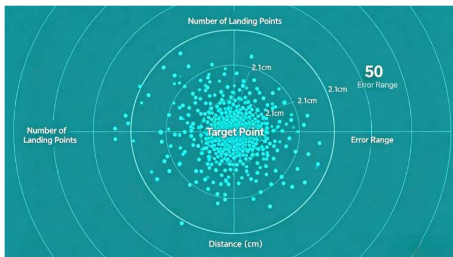
Figure 6. Distribution of UAV delivery landing errors
